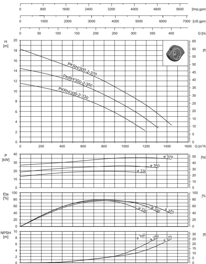
1450 min<sup>-1</sup> (400 V - 50 Hz)
