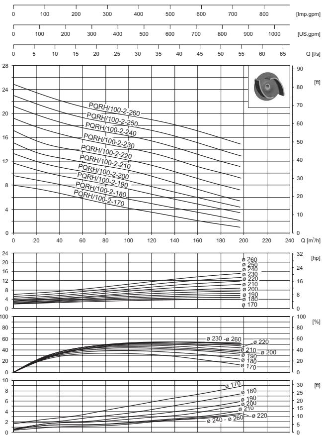
**960 min<sup>-1</sup> (400 V - 50 Hz)**
