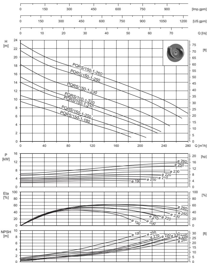
**960 min<sup>-1</sup> (400 V - 50 Hz)**
