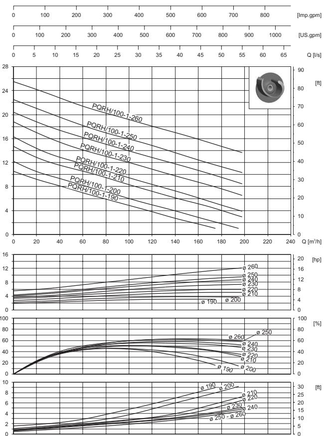
**960 min<sup>-1</sup> (400 V - 50 Hz)**
