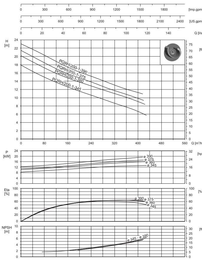
**960 min<sup>-1</sup> (400 V - 50 Hz)**
